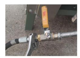
Connect the gas hose and stopcock at the inlet of the carburetor valve
