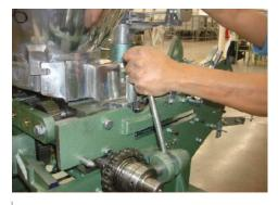
Lift the clutch lever to start recirculating the dough
