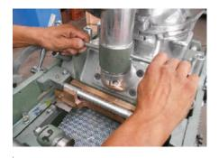
Loosen pressure chamber screws with a  $\mathsf{T}$ 20 wrench and remove the coupling.
