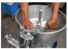
Remove the shaft support and turn assembled 18 auger counterclockwise
