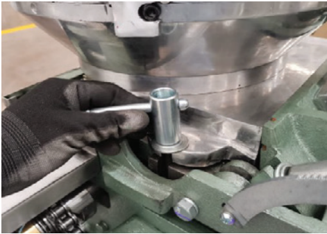
9 Loosen screws on the hopper base.
