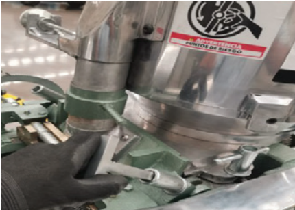
21 Tighten the pressure chamber bolts with a T spanner.
