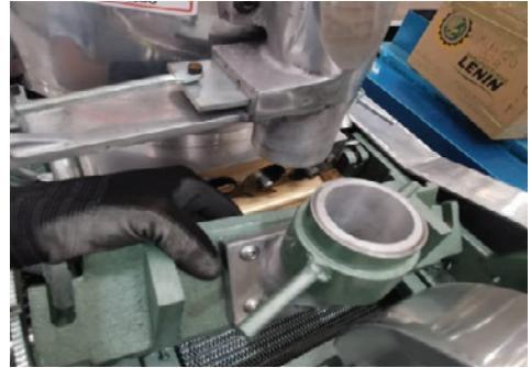
8 Remove pressure chamber.
