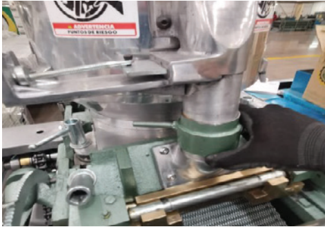
7 Remove coupling from recirculation tube.
