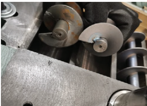
11 Verify numerical position of augers with respect to the base.
