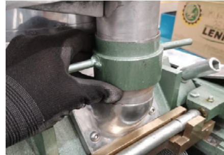
20 Place coupling in recirculation tube.
