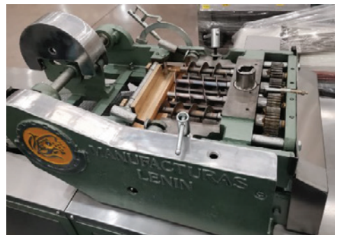
12 Lubrication in bearings, verify tightness in bearings, square, dovetail and base in general.
