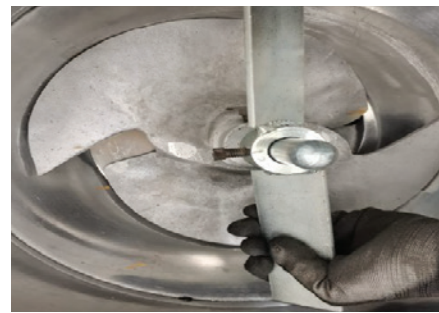
24 Rotate assembled auger clockwise.
