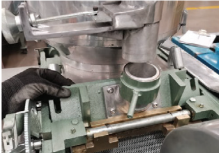
19 Place pressure chamber on the base.
