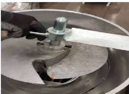
23 Place auger in hopper.
