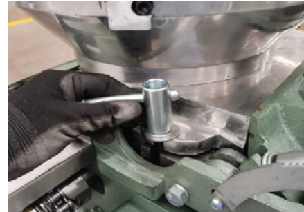
22 Tighten the hopper base bolts.
