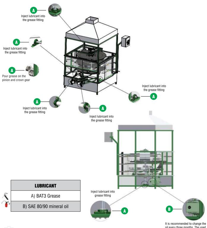
oil every three months. The used oil must be drained and 400 ml of new SAE 80/90 mineral oil must be added.
