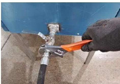
**5** Tighten with a wrench and ensure it is securely fastened
