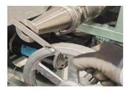
Check that the blade does not come into contact 3 with the nozzle.
