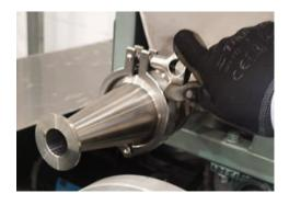
Turn the clamp screw to clamp the nozzle.
