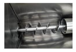
Verify the counterclockwise rotation of the cutter auger.
