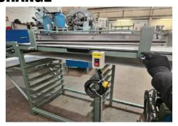
Remove the 2 retaining knobs from the base of the rail
