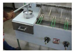
Lower the lever with the nylamid plate and apply pressure to cut the product.
