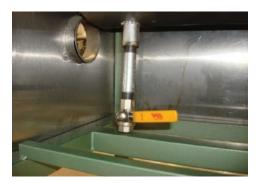
Place a 1/2" x 4" nipple and a 1/2" drain outlet at the bottom of the fryer (equipment not included).
