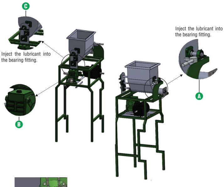
It is recommended to change the oil every three months. The used oil must be drained and 400 ml of new SAE 80/90 oil must be poured.
