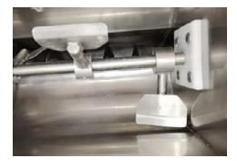
Before turning on the extruder, check that it is clean and without dough residue.
