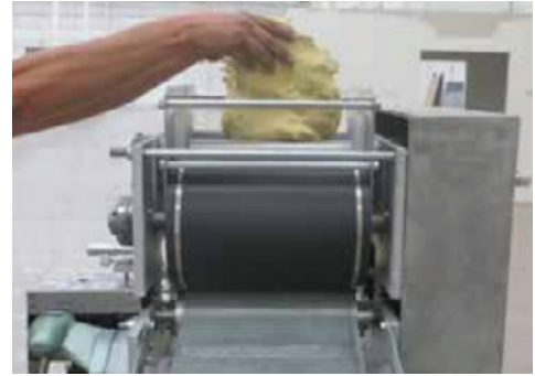
26 | Add dough to rollers manually.
