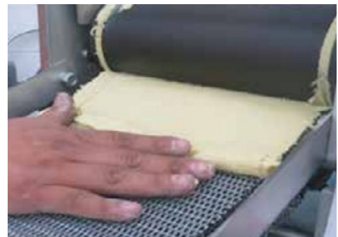
28 | Adhere curtain of dough to front roller.
