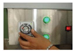
Rotate the pyrometer to 160° (35gr dough ball) The pilot lights will turn on and will turn off when the temperature is reached.
