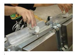
7 Verify plate temperature by placing dough ball.
