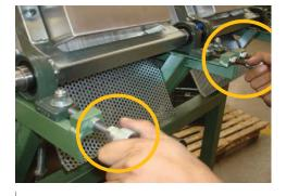
Adjust the thickness of the tortilla in the lower part by turning the knobs ONLY IF NECESSARY
