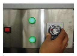
Rotate the pyrometer to 160° (35gr dough ball)
