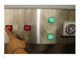
Turn on pyrometer switch (right)
