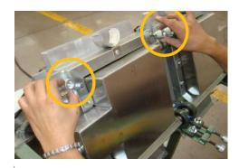
Adjust the thickness of the tortilla on top by turning the knobs ONLY IF NECESSARY
