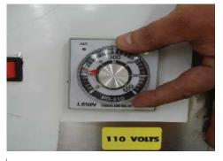
Turn the bottom plate pyrometer to 140°C, the pilot light will come on and it will go off when the assigned temperature is reached.
