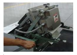
Open the plates by turning the lever to the right so that the dough falls.
