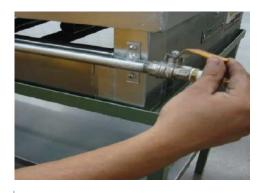
Wait for the aluminum plates to reach the indicated temperature and open the stopcock.
