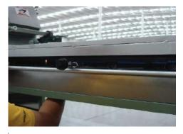
Light type H burner of the griddle and regulate the flame with the gas valve.
