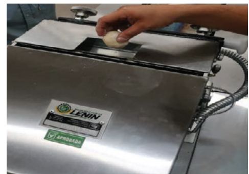
26 Place the dough ball in the groove of the upper plate of the press.
