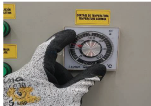
24 Turn the pyrometer to 160°C, equipment in operation indicators will light up
