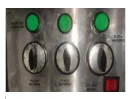
When the press is not in operation, turn off and turn the knobs to the OFF position.
