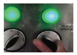
Activate second lower resistance in position No. 5, wait 8 to 10 minutes for the press to reach the appropriate temperature.
