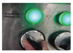
Activate the first lower resistance in position No. 5, wait 8 to 10 minutes for the press to reach the appropriate temperature.
