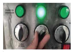
Activate upper plate in the HI (High) position, wait 8 to 10 min for the press to reach the appropriate temperature.
