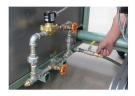
Connect gas hose to the carburetion system (factory carbureted equipment) 3
