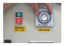
6 Rotate temperature pyrometer to 200°
