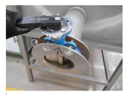
Before introducing the product in the cooker, check that the flood gate is completely closed.
