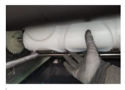
Place the cutter on the base and verify that it is correctly installed and secured
