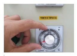
Set the pyrometer below 50°C by turning clockwise
