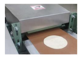
Loosen the locknut and turn the knob a little to adjust the thickness at the top of the text.
