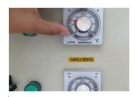
Set the upper pyrometer to 140°C by turning clockwise
