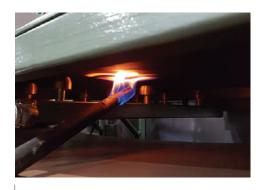
Open the gas stopcock and turn on the nozzles
