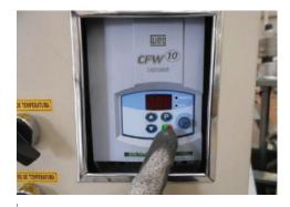
Press red and green button to turn on. With the arrows you control the speed. DO NOT PRESS THE "P" BUTTON
