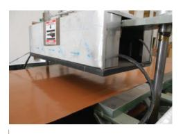
**12** Rotate the temperature control 160° on both resistances
