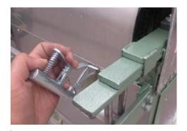
7 Regulate the teflon band tension with the ratchet
