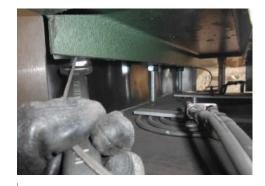
14 If necessary, adjust the uniformity of the dough, turn the interior lock nuts until level.
