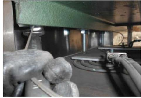
**14** Regulate the uniformity of the tortilla by turning the inner locknut until it is level.
