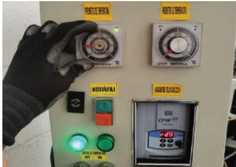
**3** Turn temperature control pyrometer #1 to 100°C for 10 minutes. Then rise to 160°C
