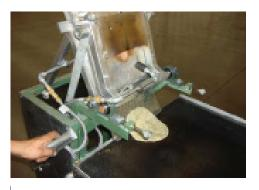
Open the plates by turning the lever to the right so that the dough ball falls out.
