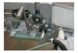
Rotate the lever continuously so that the rollers perform their function.
