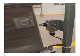
As the hopper does not have contact with the microswitch the mixer will turn off.
