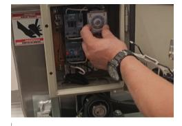
Turn the timer knob adjusting from 0 to 10 minutes.
