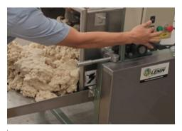
If the motor button is activated, the mixer will not work until it contacts the microswitch
