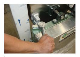
6 Turn the lever to the right to release the hopper.
